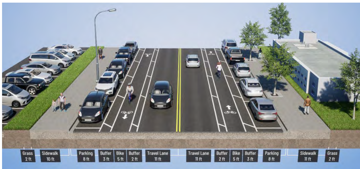
Figure 84: 3 rd Avenue Parking-Separated Bike Lanes
